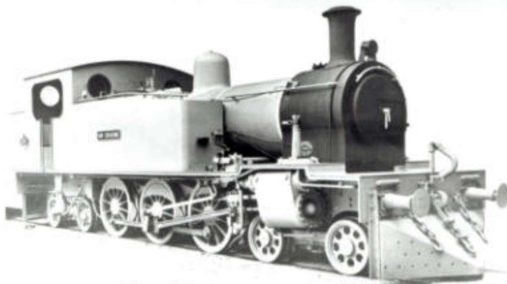
Note the Argentine-style fold-up buffers to minimise the risk of animals hit by the loco being caught in place rather than flung off to one side.
