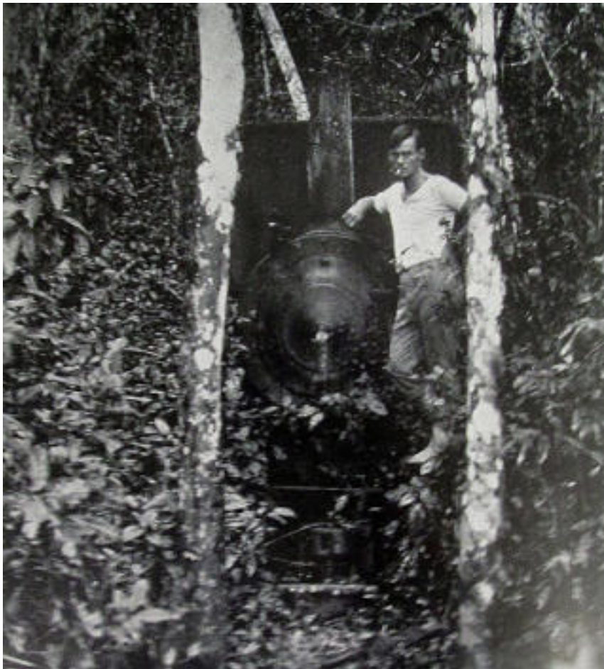
Supposedly a view of the Baldwin 2-4-4RT at Pakira Creek in the 1920s, though the cab roof looks rather different and there
