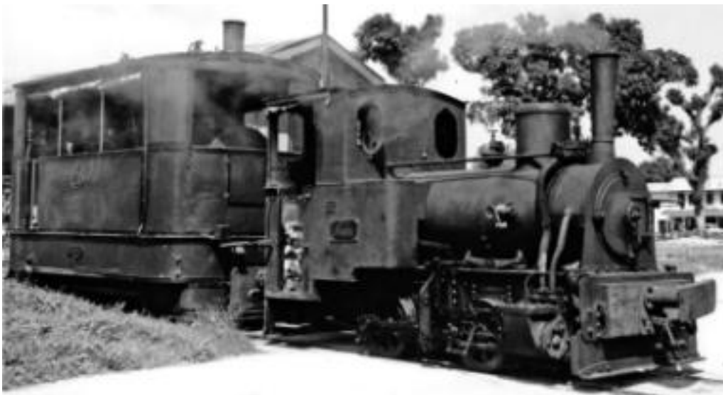
Jung 0-4-0T 'MAABO' with another of the Borsig tram engines, 5, behind. Photo from the Anthony Burgess collection uploaded to Flickr by Colin Churcher.
