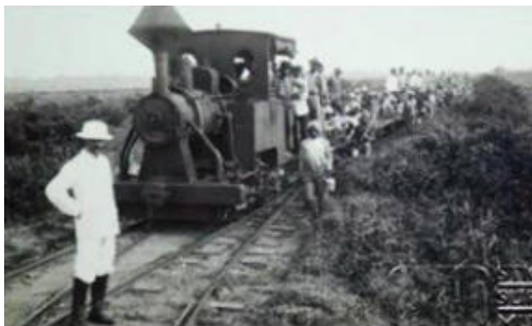
These first two pictures illustrate the same type of 0-4-0T loco, probably by Krauss or DuCroo & Brauns. The engine seen below on a train of cane, is numbered 8 on the rear cab panel and the side tank.
