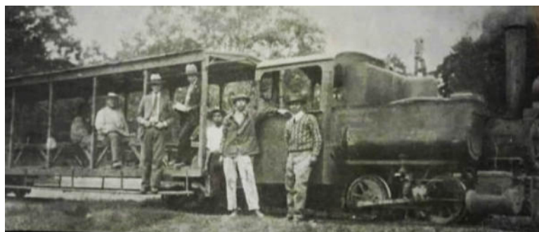
The loco above is seemingly an American built 0-4-0T though with French-style side tanks with curved bottoms, and equally clearly it is indeed shown hauling an open tramway style car.
