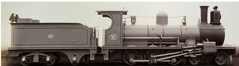
Neilson 4-6-0 no. 26 , as seen in a builders' photo. The 2-4 wheel arrangement of the tender is particularly distinctive, though by no means unique.
