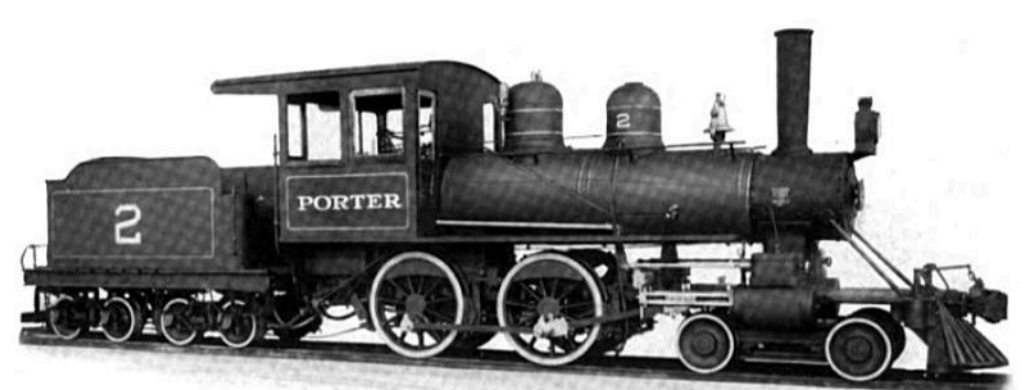
Illustration No. 2, from photograph of 10 x 16 cylinders, 36 inches gauge locomotive, exported to Central America.
