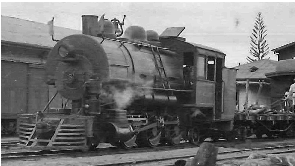
No. 15 seems to have been rebuilt as a 2-6-2ST, using the original saddle tank with a forward extension. Here is the loco in charge of a tourist train from Puntarenas to San José.
