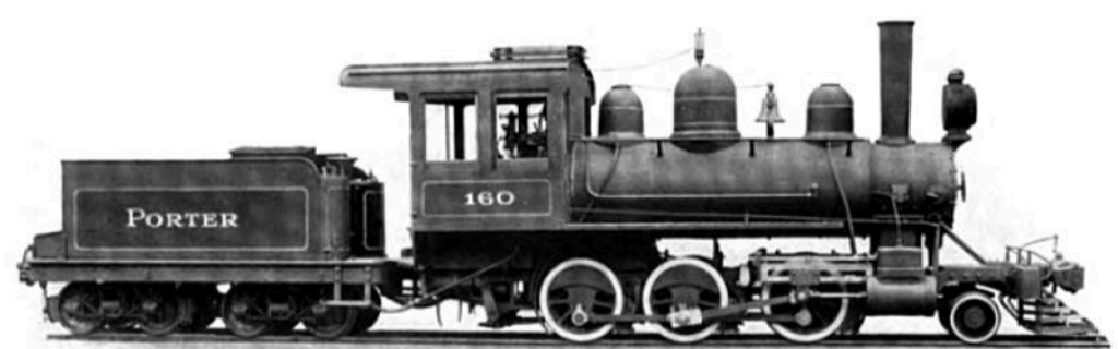
Illustration No. 160, from photograph of 10x16 cylinders, coal-burning locomotive, 36 inches gauge of track, for banana plantation in Central America
